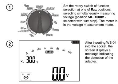
Set the measuring voltage  $V_{\text{N}}$  (applies only for **50...1000V** position of the switch), and times t1, t2, t3 as in double-lead measurement. These settings relate to the measurement of insulation resistance for each pair of leads selected in the main settings.
