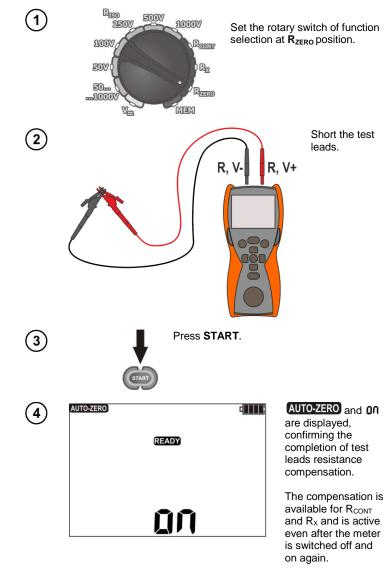
In order to remove the compensation made (and return to default calibration), perform the above-mentioned activities with test leads open – messages **AUTO-ZERO** and **On** disappear, the following message is displayed **DFF**.
