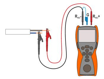
The end of the shielded cable with two banana plugs may be connected only to the meter. Do not connect it to the tested object or to the network.
